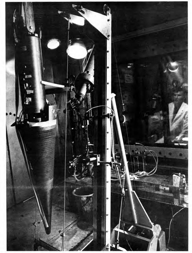
SUSPENDED from a monorail, nose cone is positioned by Dave Shirey (9321) for explosive spraying operation. He operates master-slave manipulators from behind several thicknesses of explosion-proof glass.
